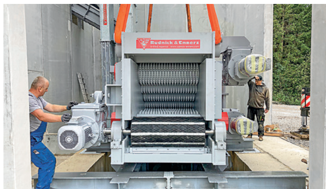
Following the good collaboration, Rudnick & Enners is currently delivering a drum chipper line for logs and cross-cut wood. In the future, the system will supply biomass for the heating plant and additional raw material for the pellet plant
