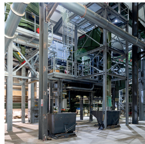
(Above) All material, boiler fuel for the CHP plant, and pellet feedstock, is trucked to the site. A JCB 560-80 Telehandler loading sawdust into the pellet plant receiving bunker. (Centre) Inside the spacious boiler house, the 4 MWth Kolbach boiler sits on raised frame. (Left) The split level pelleting line with the Stela belt dryer and CPM press on the upper level.
