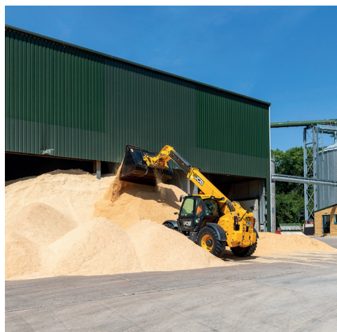
(Above) All material, boiler fuel for the CHP plant, and pellet feedstock, is trucked to the site. A JCB 560-80 Telehandler loading sawdust into the pellet plant receiving bunker. (Centre) Inside the spacious boiler house, the 4 MWth Kolbach boiler sits on raised frame. (Left) The split level pelleting line with the Stela belt dryer and CPM press on the upper level.
